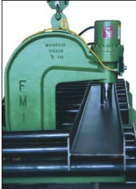
Available in 8 models, these versatile presses are primarily used for piercing the web sections of wide flange beams and channels. Plate, angles and a wide variety of structurals may be pierced in a fraction of time required by burning or drilling. Franklin assures rugged construction and offers a wide variety of punches, dies, and accessories for the presses. Versatility of applications is the element of the web series presses.
