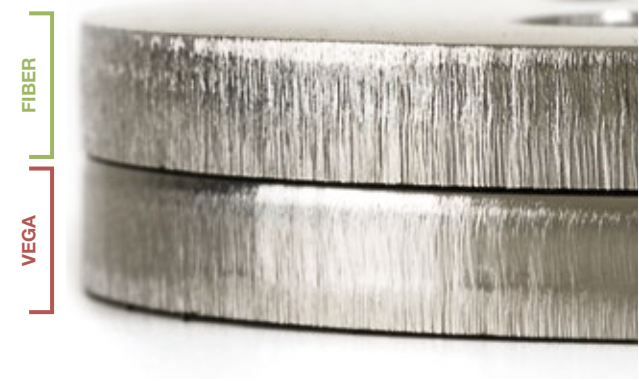
0.200" stainless steel cutting comparison between 4kW fiber laser with and without Vega feature
