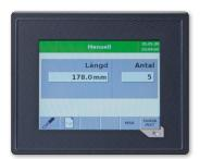
With CutLink set to Manual mode you set dimensions and the quantities. From the menu "Quick setup" you control sheet support, hold down beam and cutting sequence.
