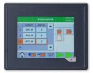
With CutLink set to Automatic mode, you can program 10 lines with different dimensions and quantities to be processed in sequence. You can save the settings in the system memory.
