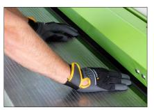
Hold down beam only 32 mm (1.25") from the cutting line for minimal waste.
